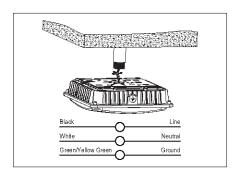
Screw the Conduit into the hole on top of Canopy light. Installation done.
