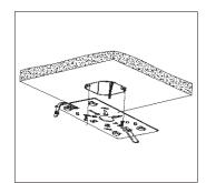
3. Attach the Canopy light with bracket by putting the ring on clips again. Connect the Black wire for Line, White for Neutral, Yellow Green for Ground.
