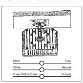
4.Slide the Canopy lights into bracket, and secure the screw on side of the light to prevent the light from sliding out from the bracket. Installation done.
