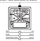
5. Replace the metal plate and the lens, make sure no wires are pinched when replacing parts.
