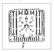
Fix the bracket on J-box, and put the wire through the central hole for wiring.
