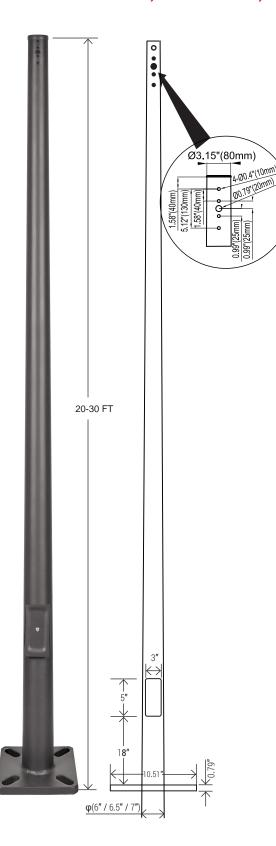
The MNW-PTR Series Round Tapered Steel poles are built from high strength steel tube and are available side drilled for arm mounted area lighting luminaires or with tenon mounts for flood and post top luminaires. Typical area lighting applications include retail centers, industrial parks, schools and universities, public transit and airports, office buildings and medical facilities. Mounting heights of 20 to 30 feet can be used based on selected luminaire application.
