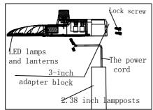
Mode 3: when the lamppost is turned into a lamppost 2.38 inches, the lamp is mounted directly on the lamp, with two screws and the lamppost fixed. The Angle of lamps and lanterns adjusts according to actual situation. Lamps and lanterns (5  $^{\circ}~$  / 2.5  $^{\circ}$ Angle 0  $^{\circ}$  / 2.5  $^{\circ}$  / -5  $^{\circ}$  ) (as shown)
