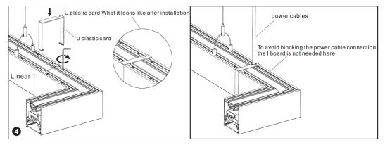
Push back Power Supply Board to Linear 1 then insert the I-shape plate to Linear 2 (or L shape, T shape, CROSS shape Combination connection fittings), tighten the I-shape plate with 8 pcs screws. Finally, the U plastic card is buckled at the joint to make the lamps and lanterns more beautiful
