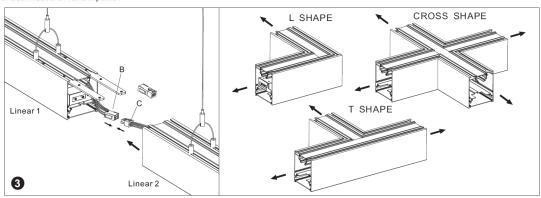
$In stall the \ Linear\ 2 \ (or\ L\ shape, T\ shape, CROSS\ shape\ combination\ connection\ fittings\ )\ to\ the\ ceiling\ and\ open\ the\ end\ cap,\ connect\ B\ and\ C\ as\ the\ picture\ shows.$
