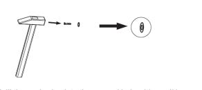
2.Drill the anchoring into the opened hole with a nail hammer
