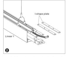
Install the Linear 1 to the ceiling as instruction of Suspension Installation. Open the end cap as the picture shows.
