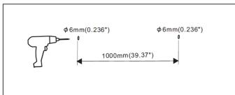
1. Drill the hole on the wall (The size is shown in the picture)
